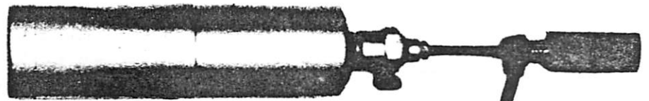
J-6084 HALIDE TORCH LEAK DETECTOR
